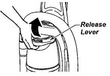
Remove dust bin from cleaner by tilting out as shown.
